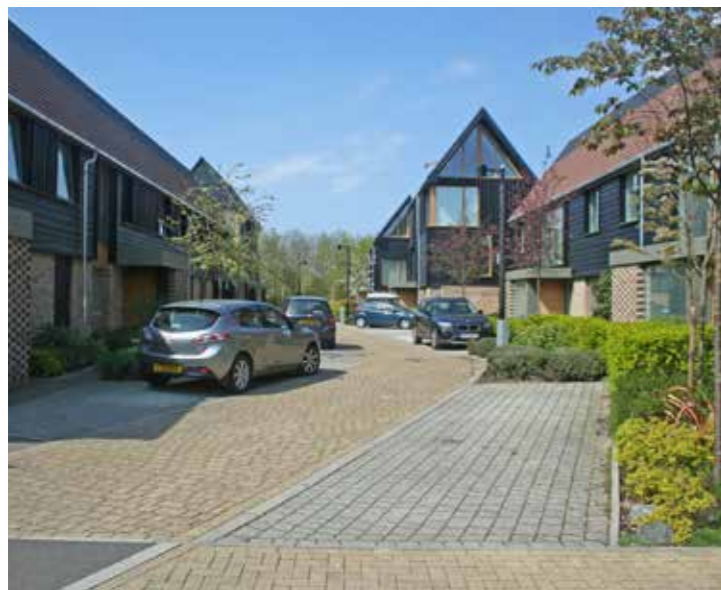
Precedent of well-designed tertiary street with minimal setback, small private strip - Abode, Great Kneighton
