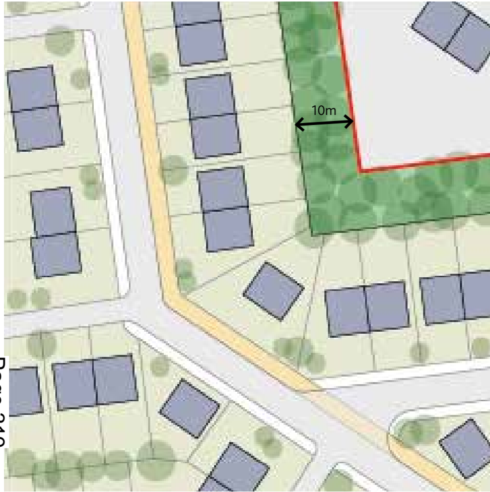
Enlarged Plan 1 - South of MU2 adjacent to existing neighbourhood to the east, where a 10m wide green setback shall be included
